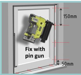
Use a pin gun that has a fine 18 gauge pin and fix at 150mm spaces. Take care not to angle the pin and shoot it out the back side. You can also use small nails, glue or double sided adhesive as other fixing options.
