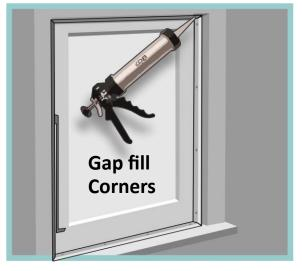
Waterbased gap filler like *No More Gaps* can be used to fill the mitre joints. Use a damp cloth to clean the area for a seamless result.
