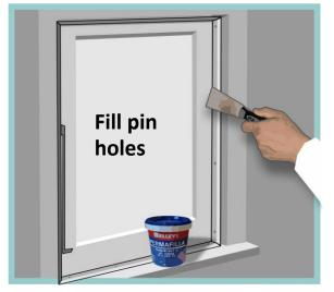
Use filler compounds, either white or brown, to fill the pin holes. Rub over them with a damp cloth to remove residue before the filler sets to avoid the need to sand.
